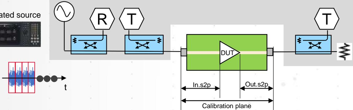
Use PNA-X “CalAll” to establish S-parameter calibration plane at DUT
