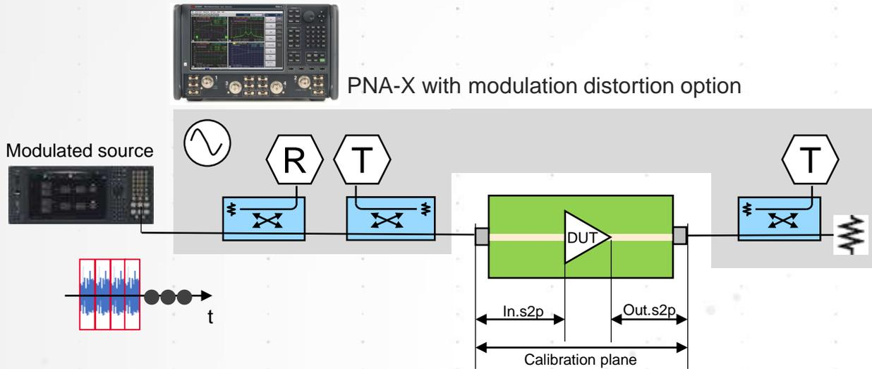
Use vector calibrated receivers to correct stimulus at DUT plane
