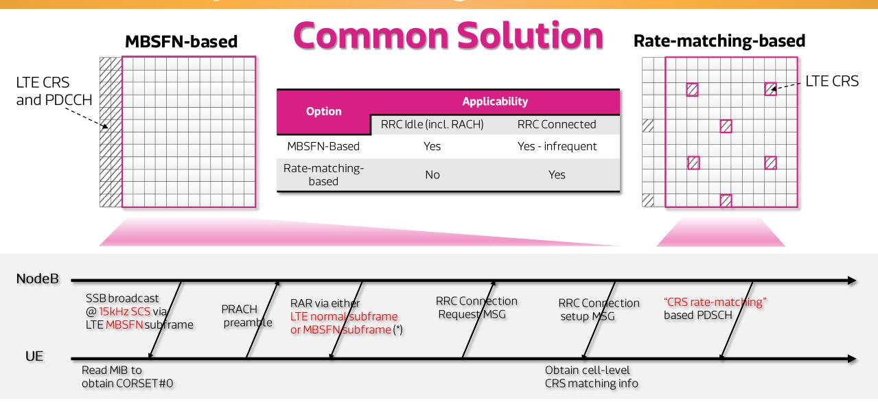
меритек \* PDSCH Type A is applied when LTE MBSFN subframe is configured. Otherwise, PDSCH Type B is applied.
